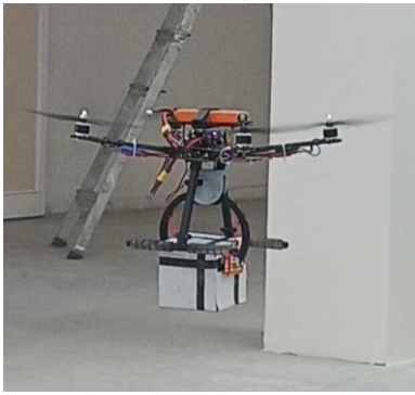
Img 1,3- Flight Training and gripper testing on drone; Img 2- Final Gripper Design
